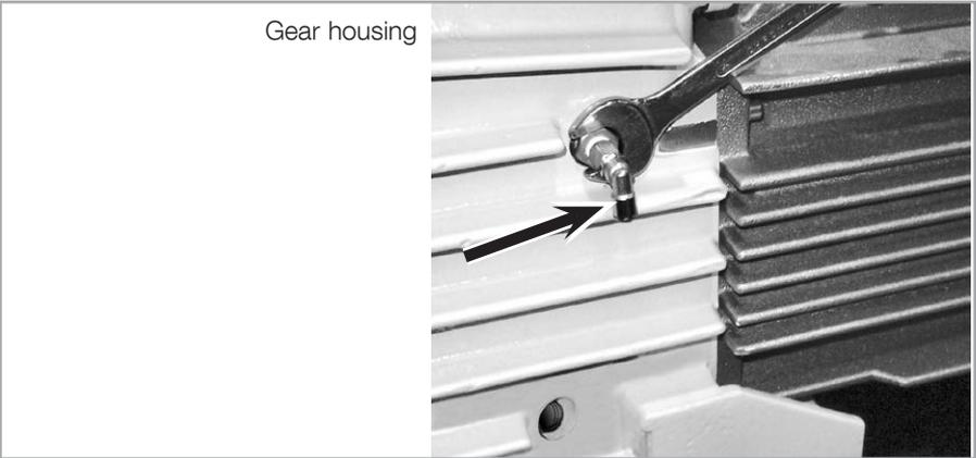
Fig. 5.5 Unscrew the throttle
